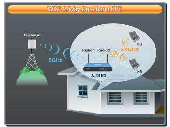
With two separate radios, A.DUO is ideal for WISP application. The 5GHz radio can be used for connection with WISP outdoor AP, and the 2.4 GHz radio is used for indoor WiFi network for home and office. Therefore, WISP no longer have to install 2 separate units to provide wireless access in subscriber's home.
