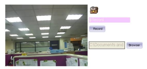
Click **Record** to activate this function. Press **Record** button to start recording. The video file is saved as ASF format into your local PC. While you want to stop it, press **Stop** to stop recording. Select **Browser**, the pop-up window to select the save path and file name prefix, select **OK** to continue.
