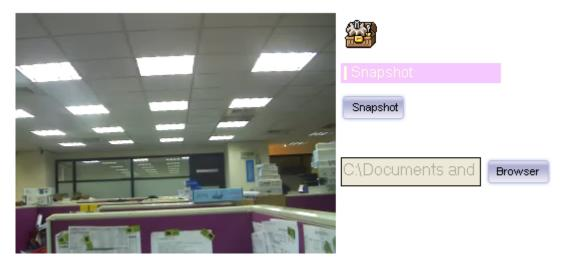
Click **Snapshot** to activate this function. Press **Snapshot** button to take a picture. The image file is saved as JPEG format into your local PC. Select **Browser**, the pop-up window to select the save path and file name prefix, select **OK** to continue.
