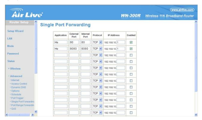
Enter valid ports in the **Virtual Server** section of your router. Please make sure to check the box on this line to enable settings. Then the device can be access from WAN by the router's WAN IP Address.
