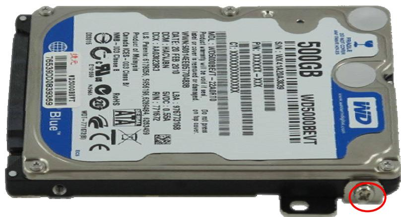
Step 3: Install 2.5" SATA HDD to the SATA connector
