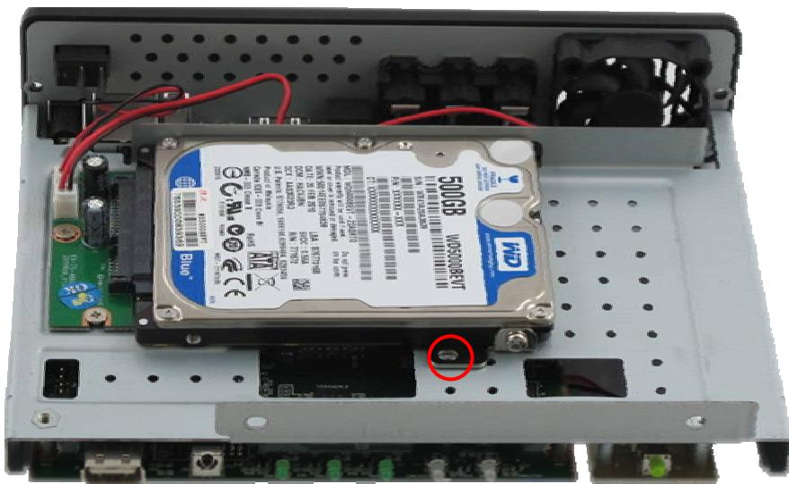
Step 5: Slide the tray back into the aluminum case and lock both screws in rear panel
