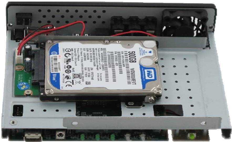
Step 4: Lock a screw to fix the hard disk mounting kit with AirMedia-350
