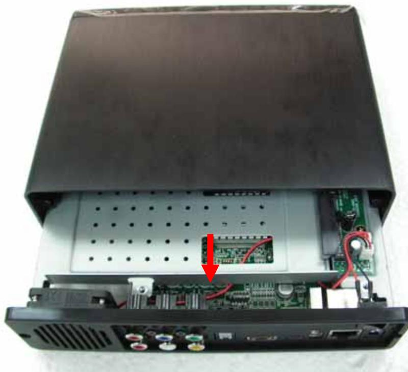
Step 2: Lock a screw to connect the mounting kit and hard disk
