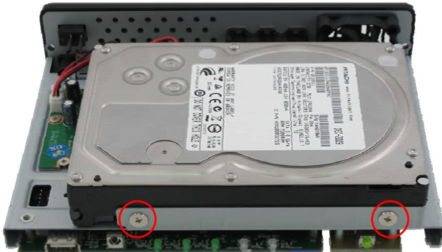
Step 5: Slide the tray back into the aluminum case and lock both screws in rear panel.
