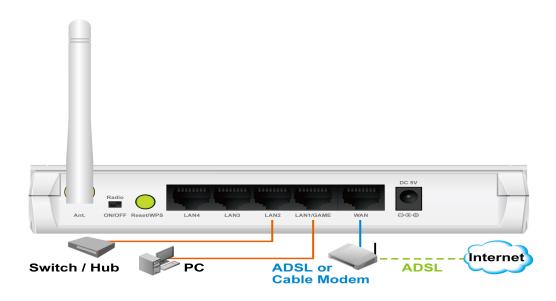
3. 4Connect the A/C power adapter to the wall socket, and then connect it to the 'Power' socket of the router.
