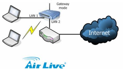
The modem is connected to WL-5460AP LAN 2 port, and client PC is connected to WL-5460AP LAN 1 port.
