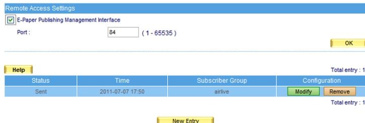
**Step8:** The port number is required for accessing the management interface from outside the internal network. The port numbers, based on the protocol is used has to be appended to the management IP address, such as <http://192.168.139.10:84>, while accessing the device remotely.
