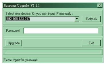
f. When you upgrade firmware successfully, please press and hold the reset button for 10 or more seconds to reset router as default setting. If the upgrade process is failed, please try again the process from step b.
