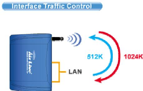
The interface QoS controls the data rate at the WLAN and LAN interfaces. Therefore, all traffics are controlled the same way. This type of traffic control is suitable when AP is used as a Client AP in "Client Mode" and WISP mode. So WISP can control the maximum data rate
