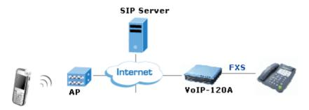
Step1: Fill the SIP account and password into the VoIP-120A and please make sure the SIP account has register success or not.
