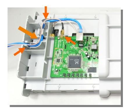
5. Now, please close the housing cover. You can now connect outdoor antenna cable to the N-Type antenna connector.
