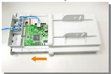
2. Remove the onboard antenna cable from the antenna connector as indicated below.
