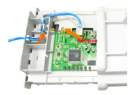
3. Now, connect one end of the converter cable(RG-316-SNF-30) to the R-SMA antenna connector
