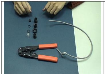
6. Assemble the component of Ethernet cable (only for WH-5000A)
