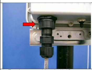
9. Turn the screw to tighten it with AP.
