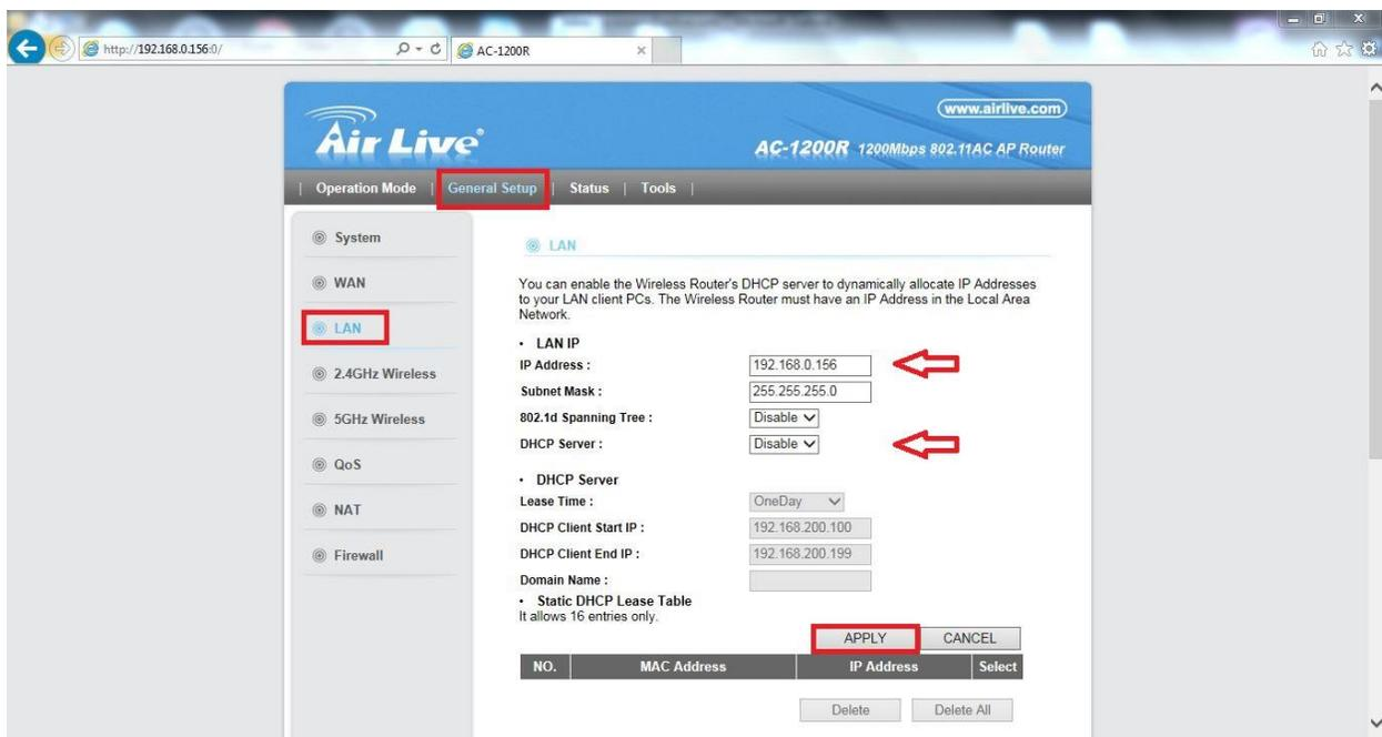
After the LAN settings have been saved, the Universal Repeater can be enabled.
