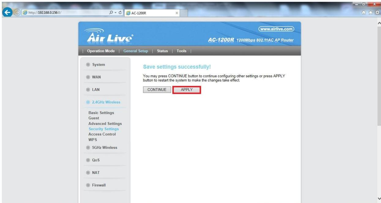
And again click “Apply” to save the settings. After the settings have been saved your AC-1200R will work as a Repeater for your main Wi-Fi router on 2.4Ghz.
