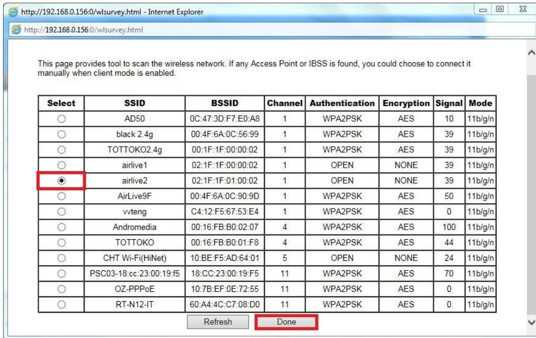
When the select wireless network has its encryption enabled a new window will open and you will be requested to enter the wireless Authentication and Encryption password. These need to be the same as those used by the main Wi-Fi router.
