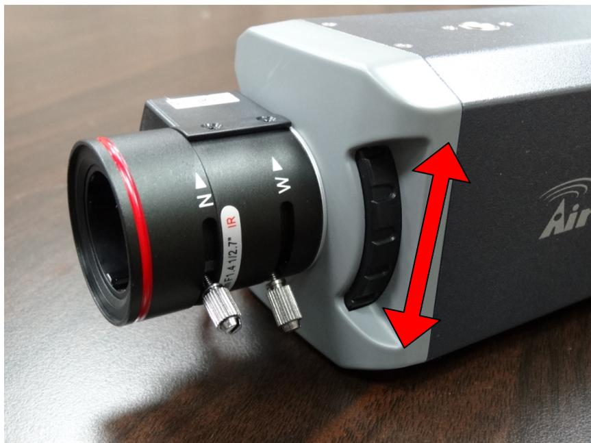
6. Enlarge the video size in the screen and adjust the lens focus until the video image is clear.
