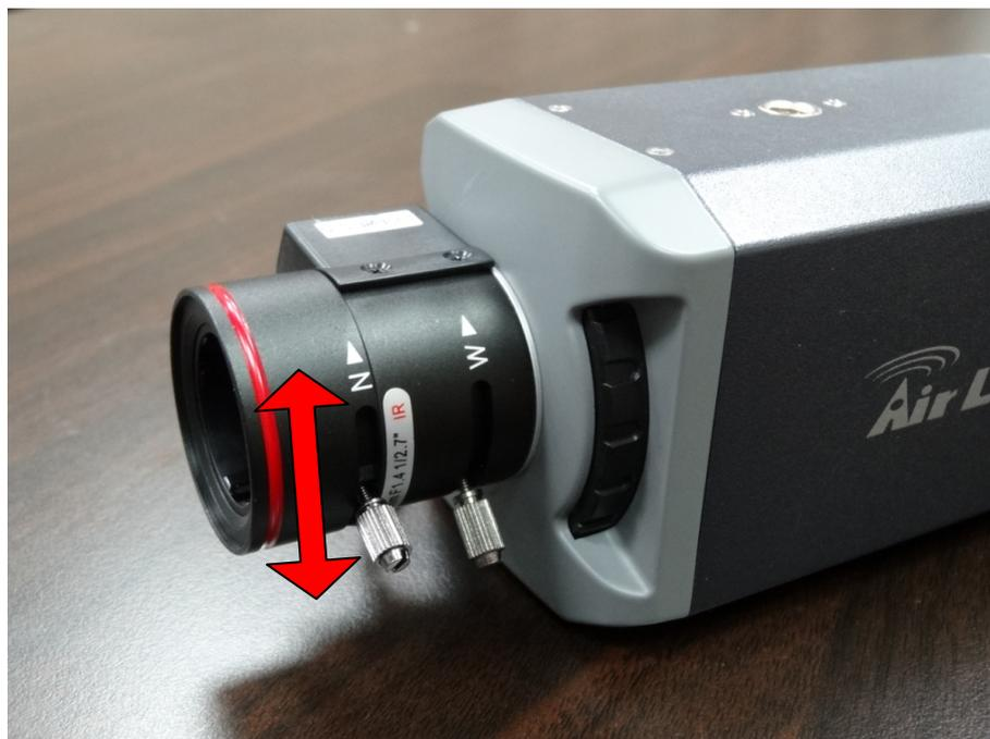
7. If the users want to adjust the zoom, they can adjust the sensor position ring and focus until the video is clear.
