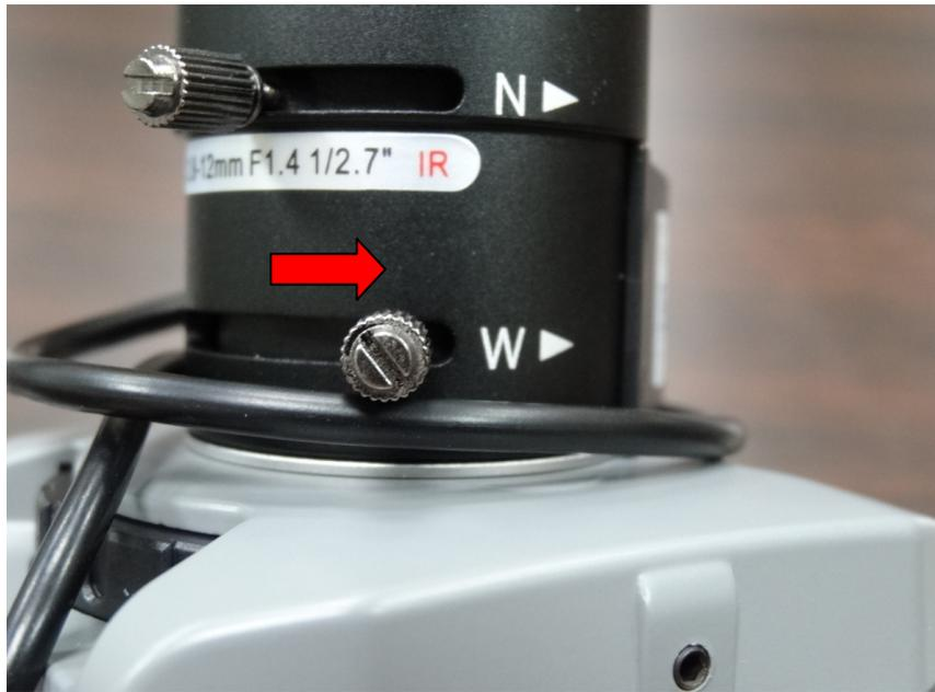
5. Adjust the sensor position ring until the video image is almost clear.
