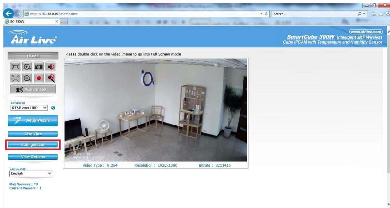
A new page will now open. On this page click on “Storage” to see the SD recording menu appear. Check mark “Recording” and Check mark “SD Card” The default file size for each recording is 55Mb you can change this also to a different value.
