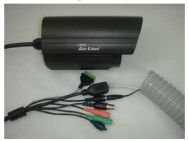
Step 3. Place all the connectors into the tube.
