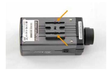
3. Remove the screws of the ACC-100 back casing.
