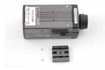
2. Drill the screws and stand onto the IP cam.
