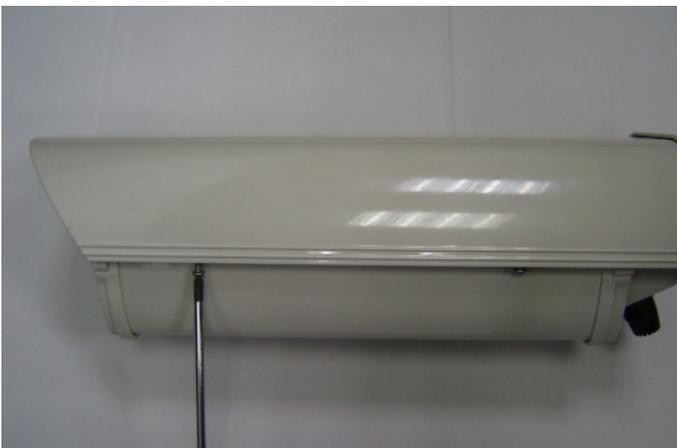
4. Open the cover and plug out the plastic plate inside the ACC-BOXCAM-IR30.
