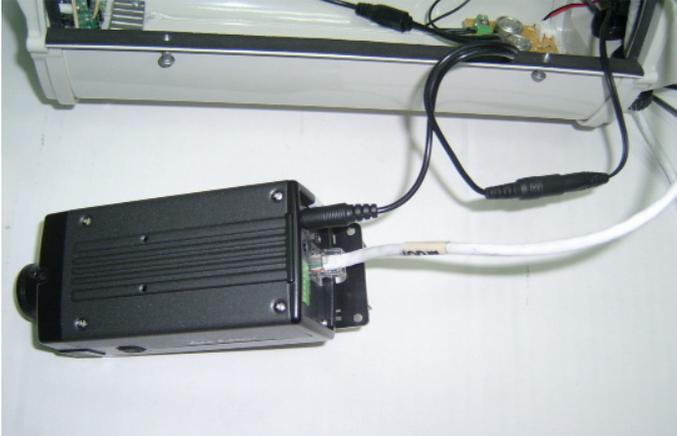
14. Pull out all the cables to the proper position and fasten the weather proof rings tight.
