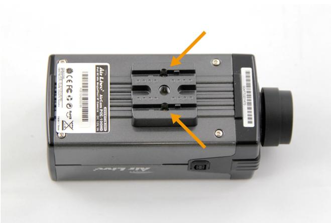
3. Loosen the screws of the ACC-BOXCAM-IR30 casing.
