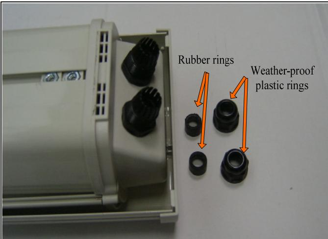
9. Insert the LAN cable(without RJ-45) and DC power cables through the weather-proof plastic ring and rubber rings.
