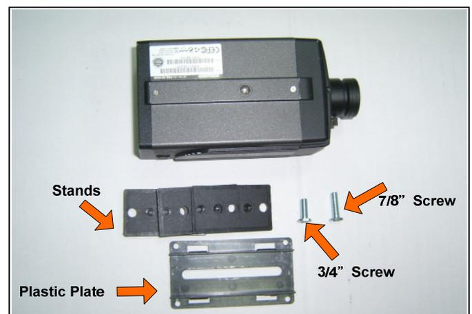
6. Fasten the 1/2" screw with plastic plate onto the IPCAM slightly
