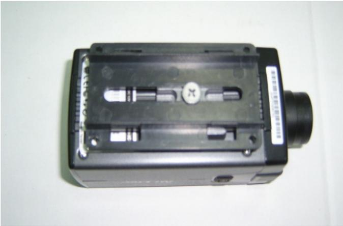
7. Move the IPCAM to the front-end of the plastic plate and fasten the screw tight.
