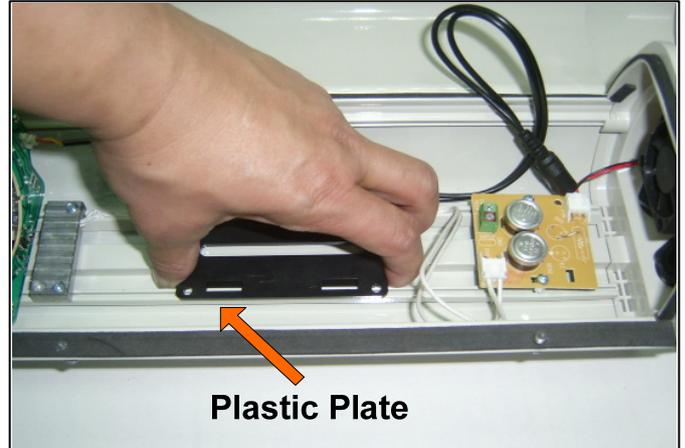
5. (1) For AirLive POE-100HD: Take out the 1/4" screws from ACC-BOXCAM-IR30 accessory bag for the POE-100HD and plastic plate as the photo.
