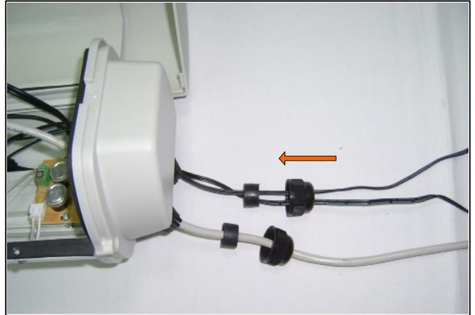
10. Install the 12V DC power for the Heater and Fan. Loosen the screws of the power socket, insert the wires into the (+/-) socket separately, then fasten the screws tight.
