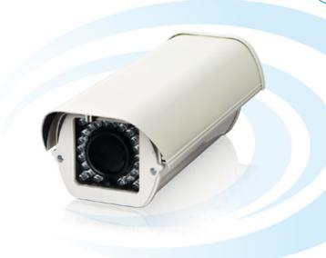
The ACC-BOXCAM-IR30 Outdoor Housing provides protection for Airlive network cameras in outdoor environment. The housing was designed to meet IP66 standard of protection, with internal heater and fan for use in cold or hot weather. The body is constructed of attractive beige color extruded aluminum.
