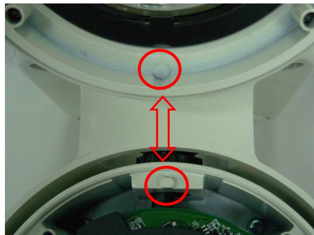
5. Put the top cover back and fasten 4 bolts back.
