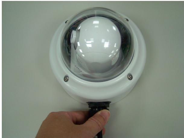
2. Unloose the cable glands body with wrench.
