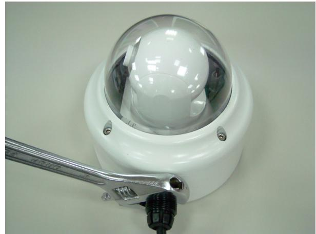
3. Remove four bolts on the case with hexagon wrench, which is in camera accessory pack.
