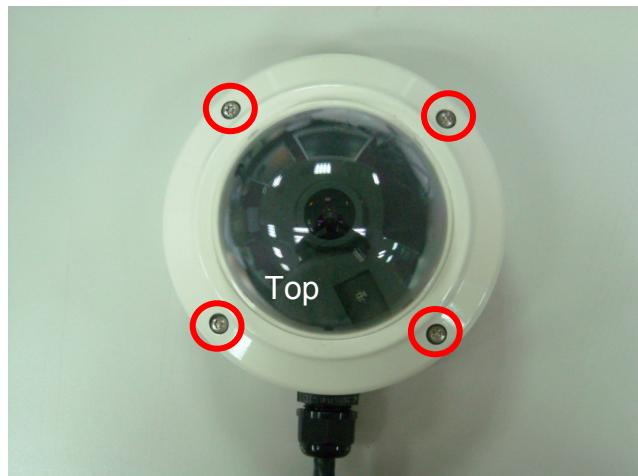
3. Fix FE-200VD on AirLive ACC-DOMCAM with four screws.
