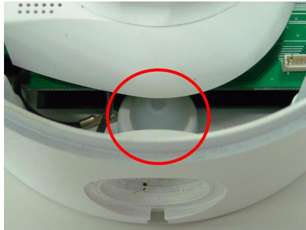
9. Let the cable wire segment go through the bottom hole from outside. Connect the wires, color to color, pin number to pin number to the PCB inside of the camera.
