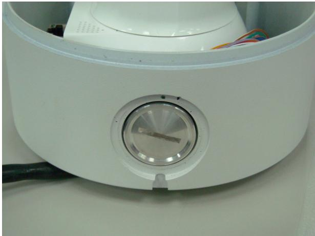
8. Remove the white rubber at the bottom of the camera.
