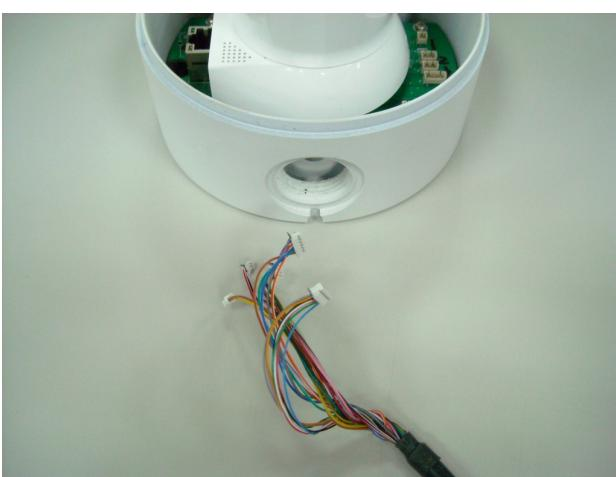
6. Remove the cable gland out of wires.
