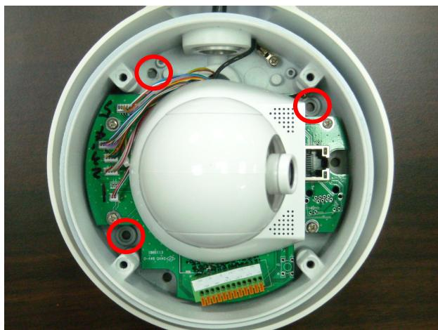
11. Place the top cover back to original position and fasten with 4 bolts.
