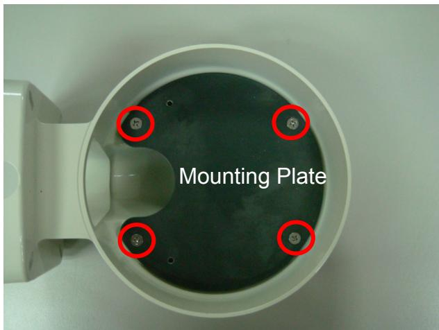
2. Remove four bolts to take FE-200VD top cover out with hexagon wrench which is in camera accessory pack.
