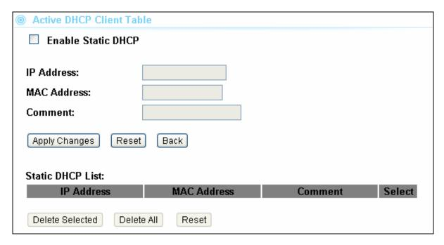
If you want to lock IP address to a MAC address, you should add DHCP clients to the "Static Lease Client". Up to 40 entries can be entered. Below is the procedure for adding an entry:
