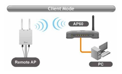
In Client Ad Hoc mode, AP60 can connect to other wireless adapters without access point. Users can attach a computer or a router to the LAN port of AP60 to get network access.
