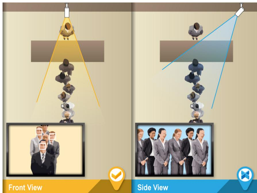
Note: The minimum distance is for reference only. This number is tested base on ACC-MPL-2812 v2 with 2.8mm Focal Length. Difference Focal Lens may have difference appropriate camera height.
