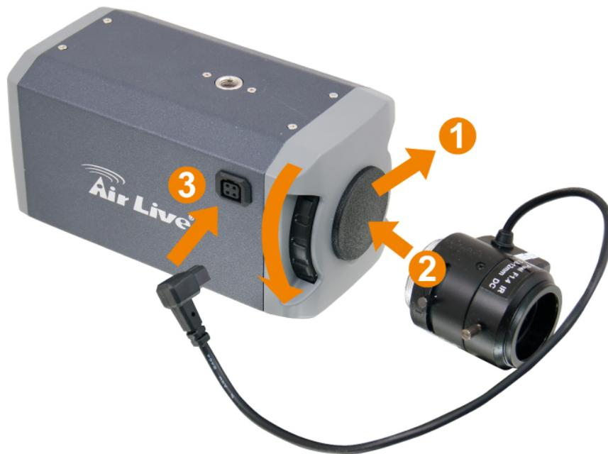
When you use a DC-Iris lens on your camera, you can adjust the brightness of the video image through the Iris Level screw-knob on the back panel of the camera.
