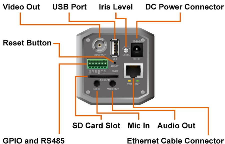
**1. RJ45 LAN socket:** Connect to PC or Hub/Switch.
