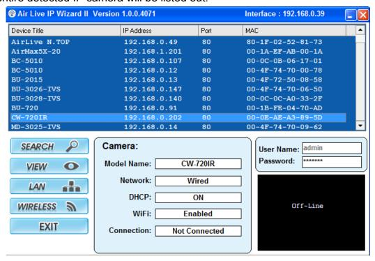
5. If the Camera's IP address is in the same IP segment as your LAN, select the founded IP Camera and double click on the item. Then, the default browser will show up and connect to the IP camera's Web automatically.
