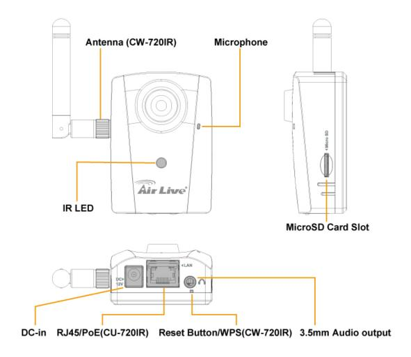
1. RJ45/PoE (CU-720IR) socket: Connect to Hub / Switch / PC.
