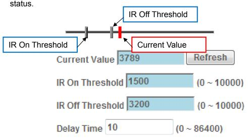
Delay Time: Select the time delay of the ICR switching.
