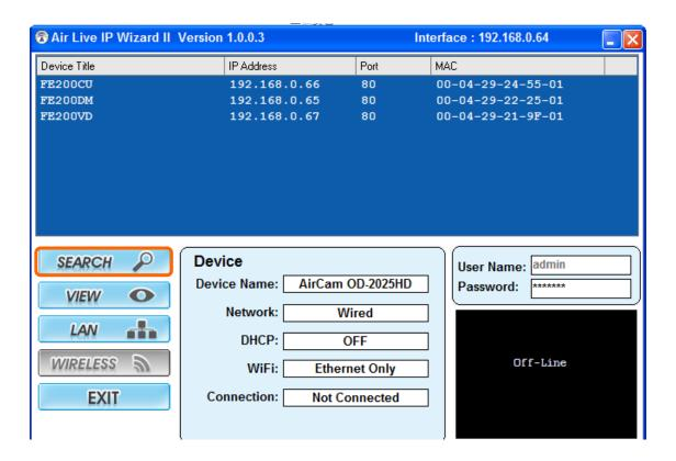
When launch the IPWizard II, a searching window will pop up. IPWizard II is starting to search Network Cameras on the LAN. The existed devices will be listed as below.
