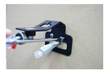
3. Install the FE-200CU onto the stand, and connect the network cable.
