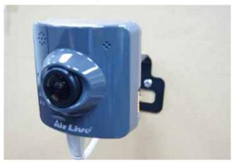
4. You can adjust the silver screw to fix the angle of camera.
