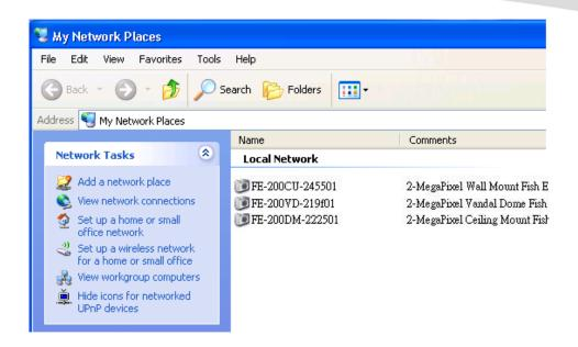
Click the targeted **Device**. Then Internet Explorer will connect to this Network Camera automatically.
