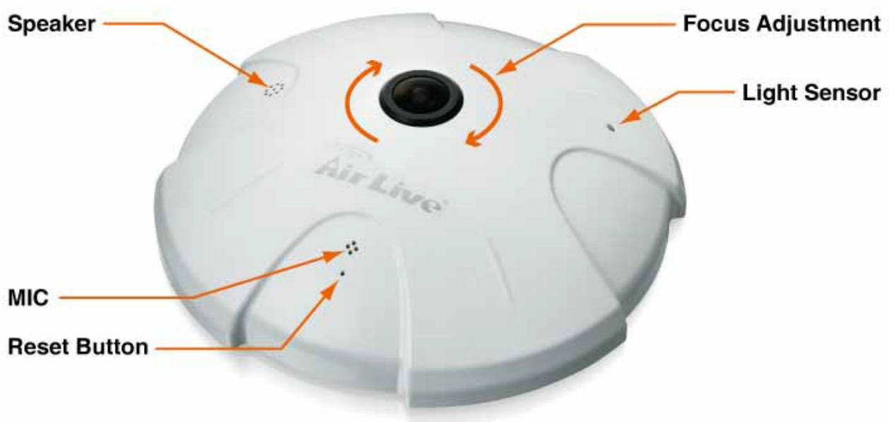
1. Light Sensor: The Light sensor is for detecting IP Camera environmental illumination, and if IP Camera was in the dark/night environment, IR Cut Filter is switched off to let infrared light pass through for clear night view.
