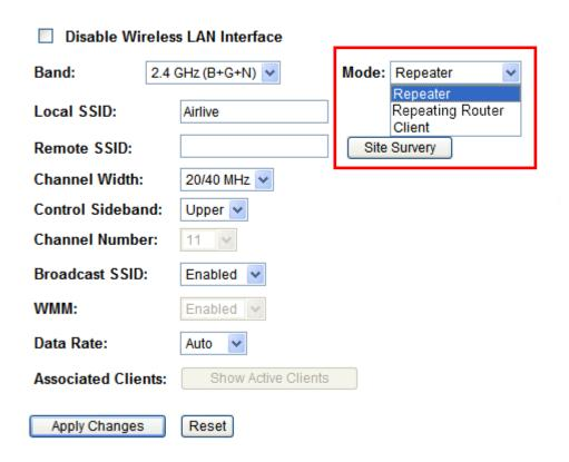
If set to Repeater (**Client**) mode, If set to Client mode, this device can work like a wireless station when it's connected to a computer so that the computer can send packets from wired end to wireless interface.
