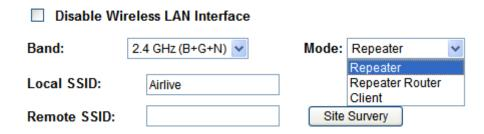
In Repeater Mode, there are three sub modes, Repeater, Repeating Router and Client mode. According to different sub mode selected, the web will be slightly different for user to do the proper setting. Because in the repeater mode, the wireless setting will be mostly the same the upstream Router or AP, if not necessary, we recommend you to use the site survey or WPS function for getting these values automatically.
