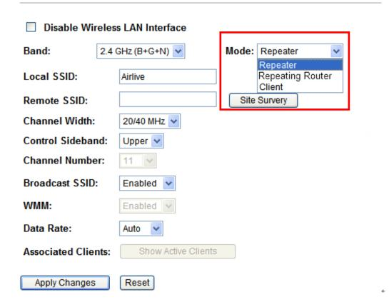
If set to Repeater (**Repeating Router**) mode, In Repeating Router mode, the AP will behave just the same as the Client mode for wireless function. However, Router functions are added between the wireless WAN side and the Ethernet LAN side. Therefore, the ISP Subscriber can share the Repeating Router connection without the need for extra router
