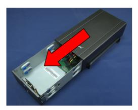
• Install the first hard drive by placing it in the enclosure and connecting the SATA plus power cables.
