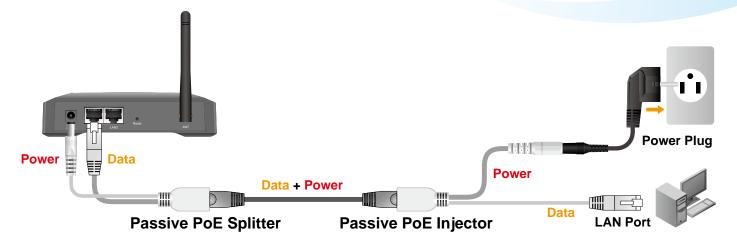
\* Passive POE has shorter cabling distance. For longer cable distance up to 100 meter, please check AirLive's 48V 802.3af PoE products.
