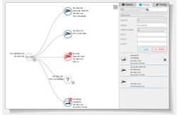
VLAN is an important function to put devices on the same network group. But configuration is always a complicated procedure. The AirLive Topology switch features graphical VLAN which let you choose which devices to be on the same VLAN group from the topology diagram
