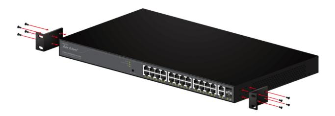
B. After attached mounting brackets, position the POE-GSH2624-370 in the rack by lining up the holes in the brackets with the appropriate holes on the rack. Secure the POE-GSH2624-370 to the rack with a screwdriver and the rack-mounting screws.
