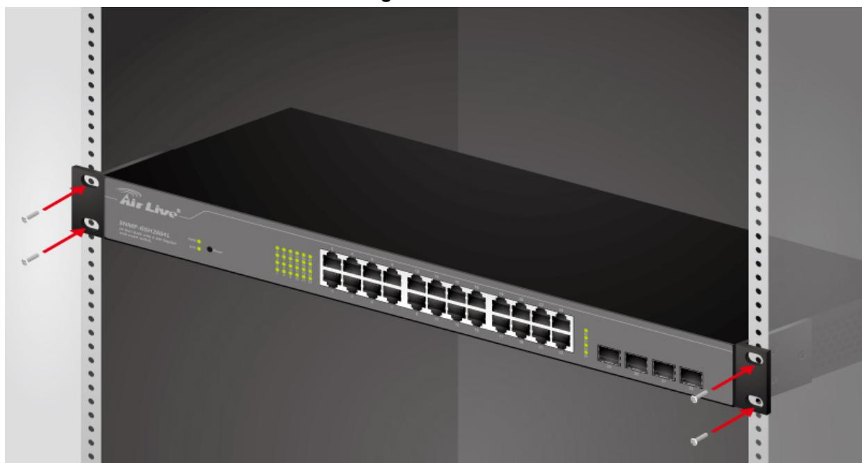
Attaching the Switch to a 19-inch rack
