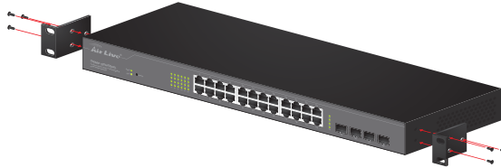
Fastening the brackets on the Switch
