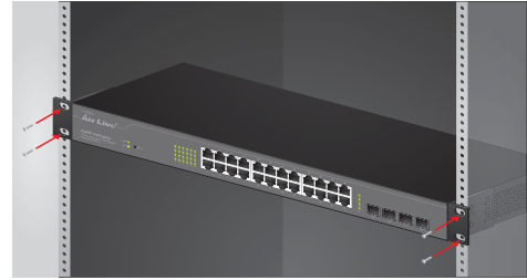
Attaching the Switch to a 19-inch rack
