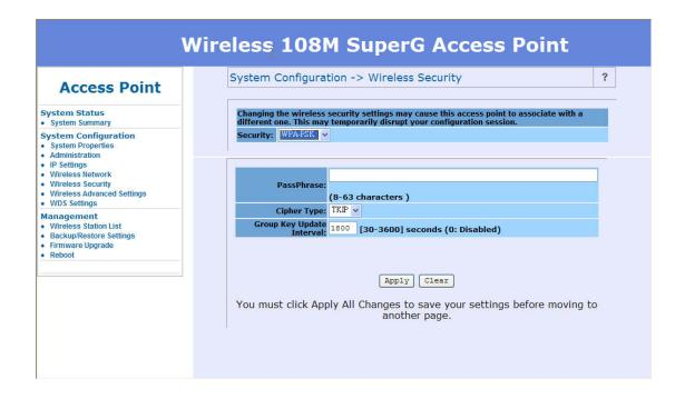
WPA option features WPA used in coordination with a RADIUS server. (This should only be used when a RADIUS server is connected to the Access Point.)
