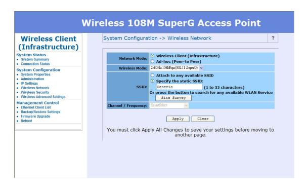
The Site Survey page can help you identify all the APs currently working in your environment. Just easily click on the BSSID column, the system will join you to the SSID you specify. In the Site Survey page you can also see the details of all SSID currently available.
