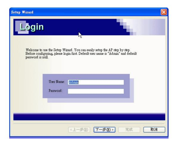
After type in correct user name and password, the utility will lead you into "**IP Setting**" page. Here you can choose to get IP from a DHCP server or specify IP address manually. Choose to obtain an IP address from DHCP server if your environment or ISP provide DHCP server. Otherwise, you can manually setup IP address. Keep the default IP setting if you are not familiar with TCP/IP setting. After you finish IP setting, click on "**Next**" to continue the configuration.
