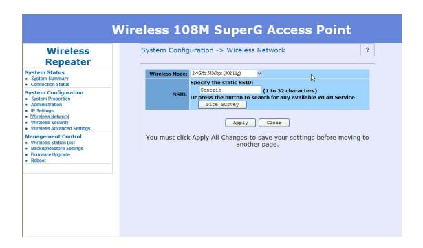
After click on the "**Site Survey**" button, you can choose the Access Point you need to extend its range by clicking on "**BSSID**" column. Then "**Apply**" the change to make sure system working properly with new setting.
