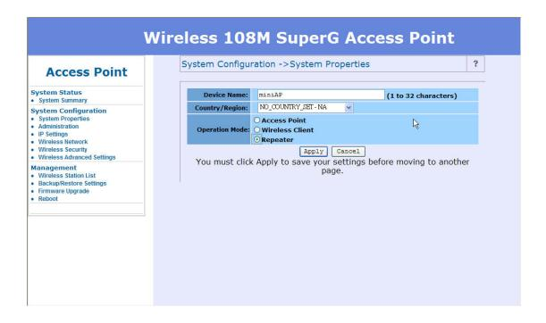
After enable the repeater mode, you can click on "Wireless Network" and choose "Site Survey" to pick one of the SSIDs you would like to retransmit its signal. (Please be awarded that while using the repeater mode, the throughput performance maybe nearly only half compare with access point mode. Because the repeater needs to communicate with original AP and also the clients associate to the repeater at the same time.)
