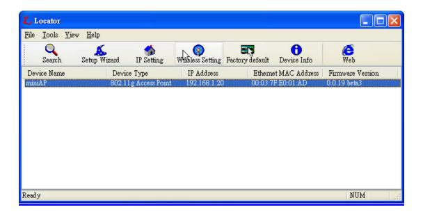
To setup the access point, just simply click on the "**Setup Wizard**" icon and the Locator configuration utility will lead you step by step to finish all the settings. After click on the "**Setup Wizard**" icon, the first page show up will be "Login". Please input your user name and password into the column. Default user name and password ex-factory as below:
