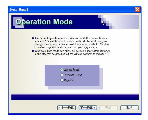
Here we choose the AP to work in Access Point mode, and then the utility will ask for SSID, Channel and Wireless Mode. Keep the default value if you do not have special requirement for these settings.
