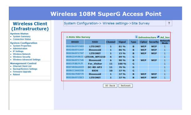
After you determine which AP (SSID) to join, you can click on the BSSID column your want to choose. The system will automatically join the SSID you specified
