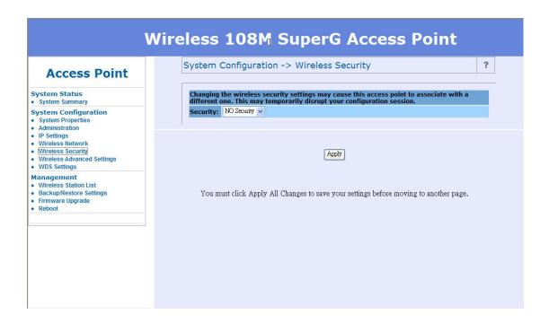
WEP is a basic encryption method, which is not as secure as WPA. To use WEP, you will need to select a default transmit key and a level of WEP encryption,
