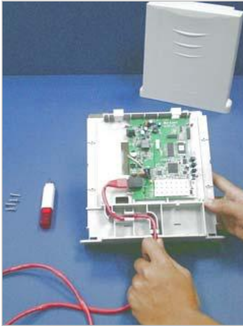
Step 5: Put the Ethernet cable along the module, till the exit (at the bottom of Housing).
