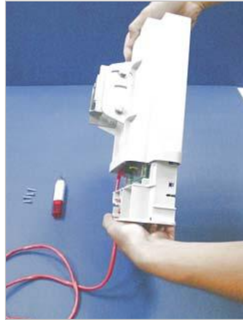
Step 6: Make sure that the other side of Ethernet cable is out of housing. Close the housing.
