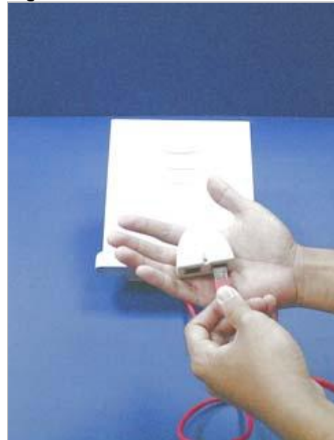
Step 8: Plug the Ethernet to the PoE "P + DATA OUT" jack of injector.
