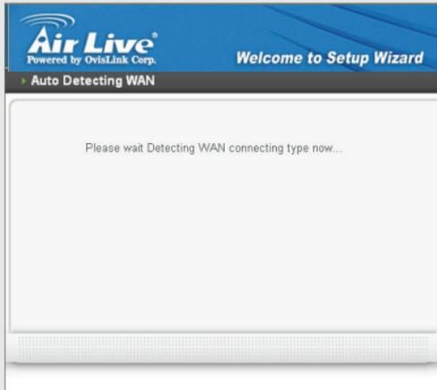
If the WLAN Router is unable to auto detect your Internet connection, you will need to manually select the Internet connection type: Obtain IP automatically; Fixed IP, PPPoE, PPTP, L2TP or BigPond.
