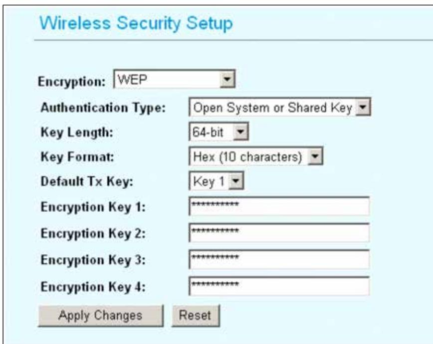
configure up to 4 keys using either ASCII or Hexadecimal format.
