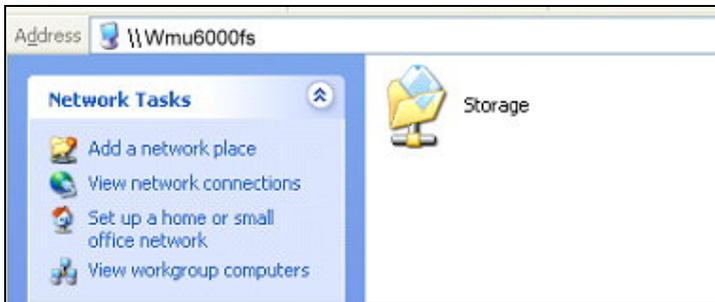
Click the **“Storage”** icon, and will find the **C folder** as below. This means you are successfully connected to the **AirLive WMU-6000FS** storage function.
