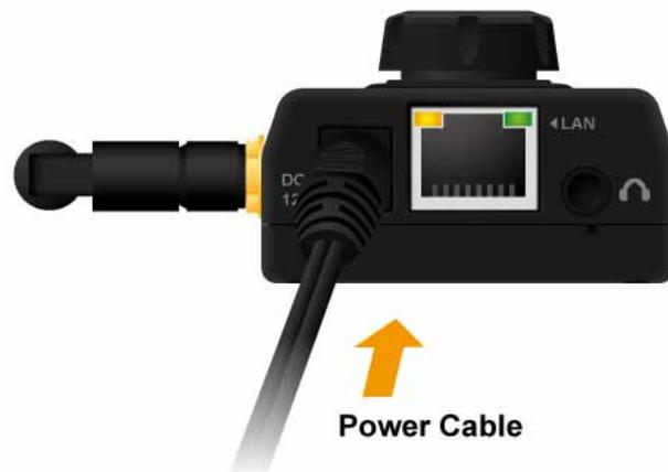
Once you have installed the Network Camera well and powered it on, the network accessing type LED will turn on. It means the system is booting up successfully. Furthermore, if you have a proper network connection, and access to the Network Camera, the LED will flash green under wired mode or orange under wireless mode.
