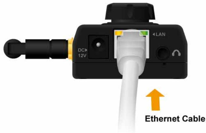
4. Connect the external power supply to Camera Connect the attached power adapter to the DC power jack of the Network Camera.
