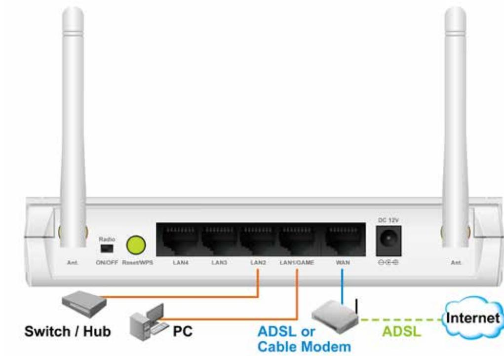
3. Connect the A/C power adapter to the wall socket, and then connect it to the 'Power' socket of the router.
