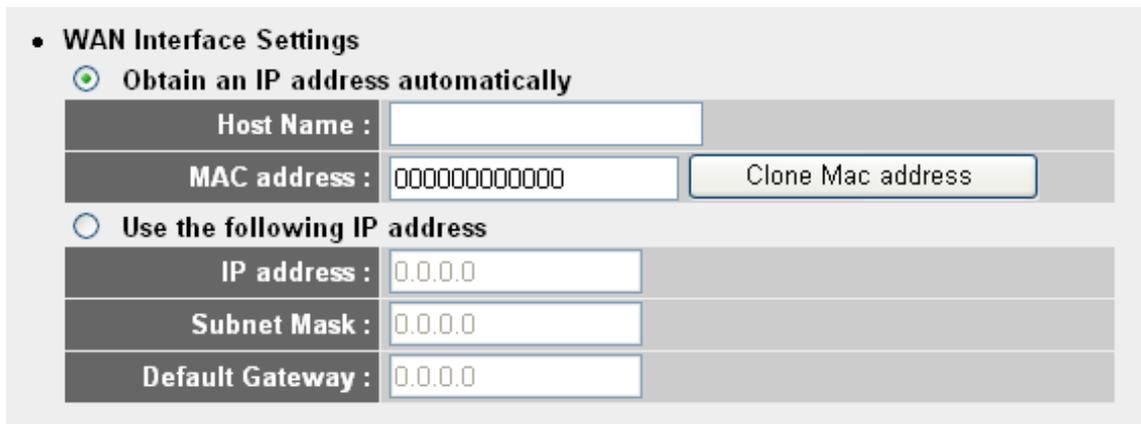
The screenshot shows the 'WAN Interface Settings' section of a configuration interface. It features two radio button options for IP address acquisition. The first option, 'Obtain an IP address automatically', is selected. Below it are fields for 'Host Name' and 'MAC address' (with a 'Clone Mac address' button). The second option, 'Use the following IP address', is unselected. Below it are fields for 'IP address', 'Subnet Mask', and 'Default Gateway', all containing the default value '0.0.0.0'.
